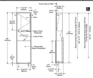
Rough Wall Opening 16" (405mm) wide 54-3/4" (1390mm) high 7-5/8" (195mm) minimum recessed depth
